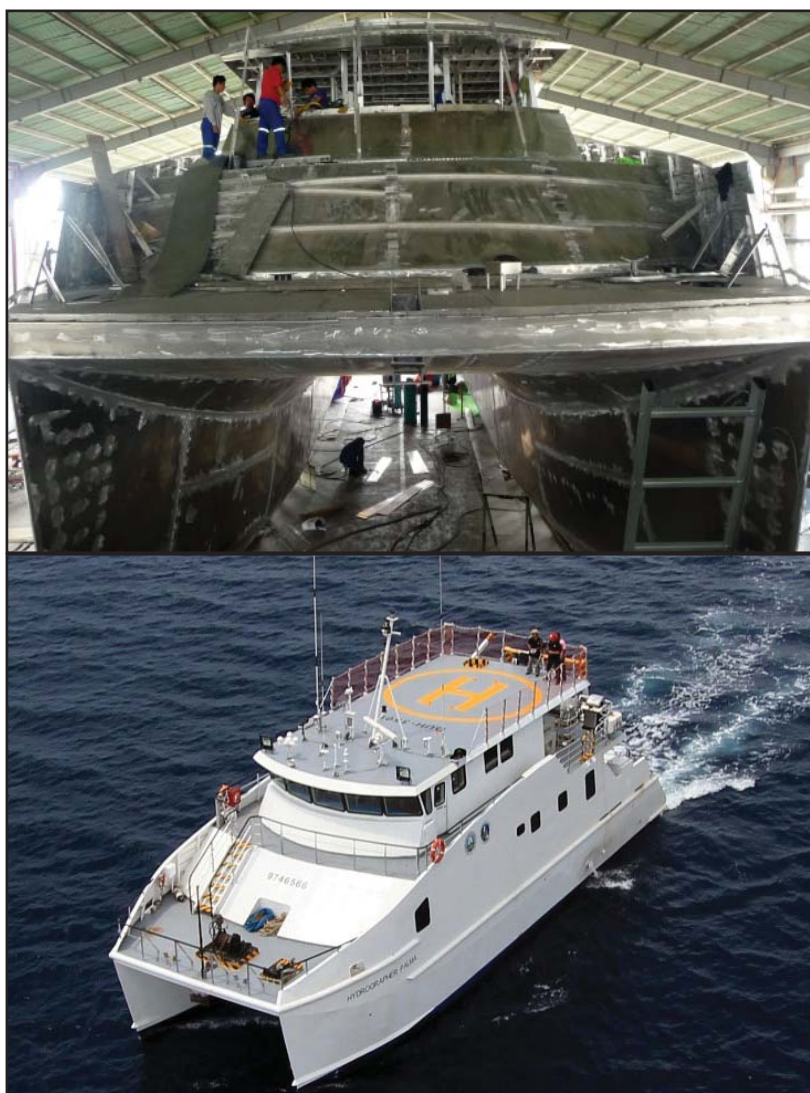
23-Meter Hydrographic Aluminum Catamaran boats built for the National Mapping and Resource Information Authority of the Philippines by Colorado Shipyard Corp. Photo Courtesy of: Colorado Shipyard.
