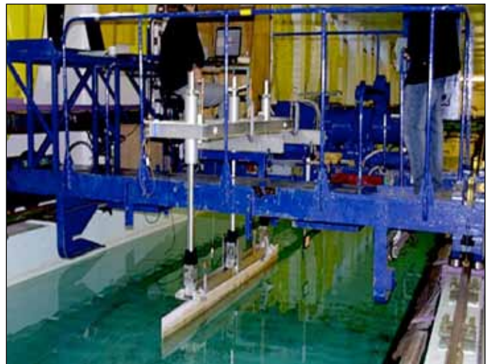
Figure 1. Tank Testing Basin with Scaled Ship Model
