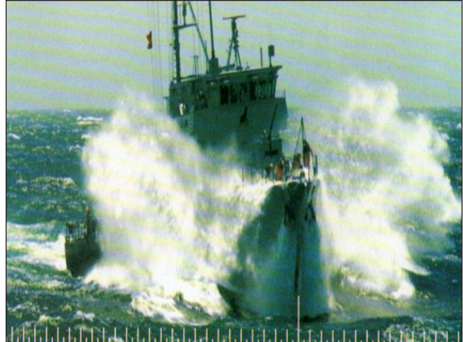
Fig. 3: Frequency of deck wetness (submergence of main deck forward) can be felt 540 times per hour.
