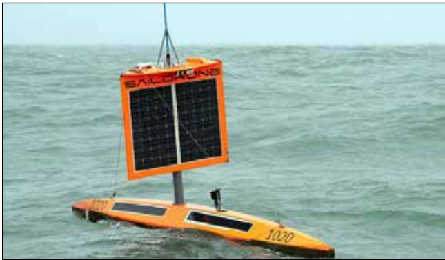
The top of the wing to the bottom of the keel is loaded with science sensors.
