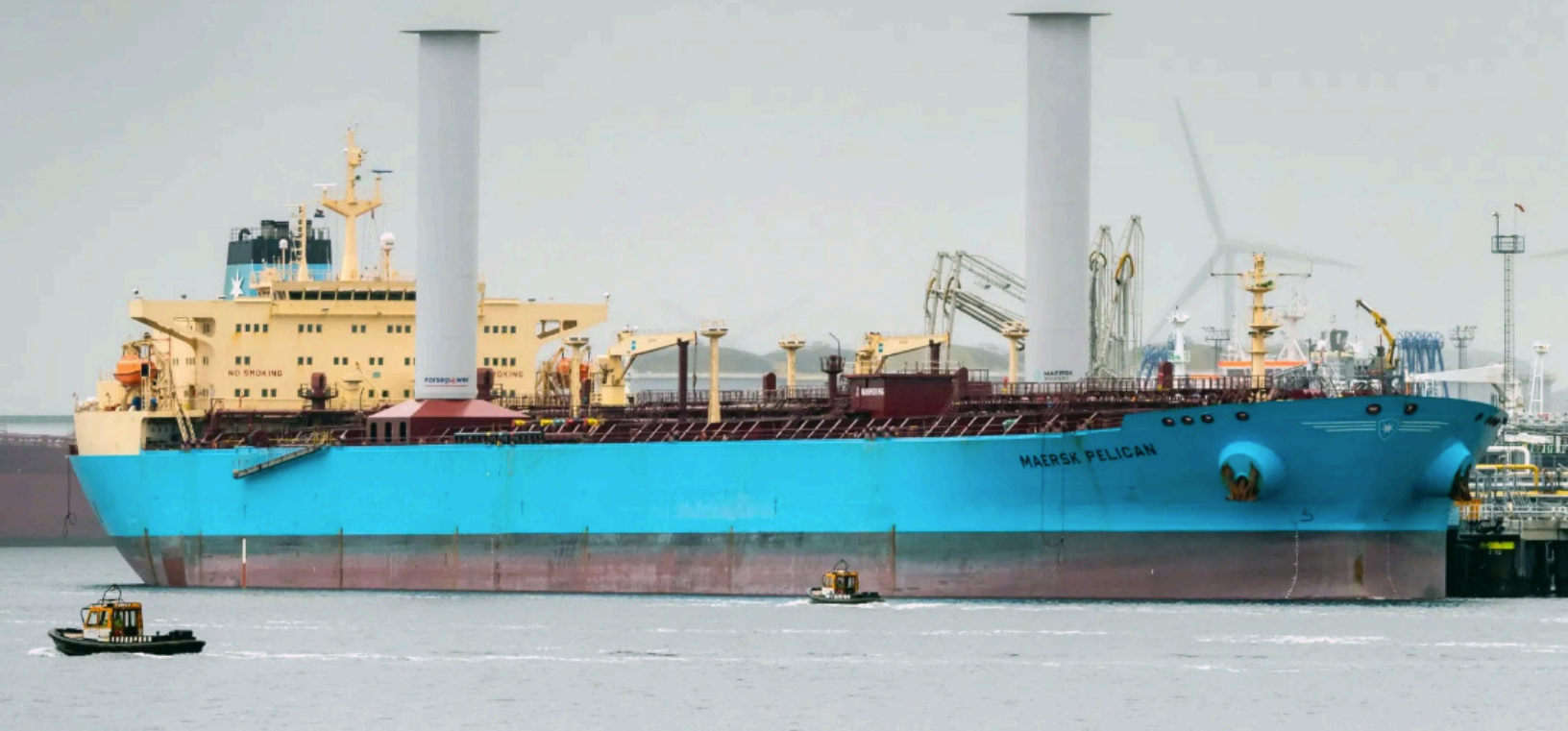
The Maersk Pelican was fitted with two 30m high Norsepower's Rotor Sails. Photo courtesy of Maersk.
