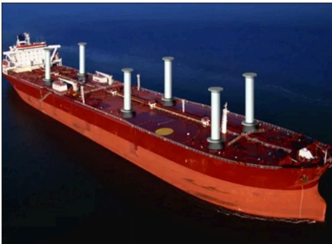
Norsepower's Rotor Sails. Image courtesy of Norsepower.
