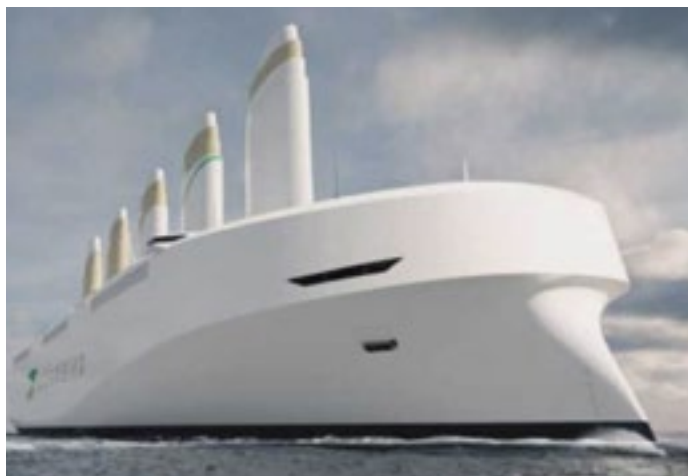
The engineless modern cargo transport sailing ship Tres Hombres. Image courtesy of Fair Transport. Sails that don't look like sails: Wallenius Marine is developing the Oceanbird, able to ship 7,000 cars and trucks across the Atlantic propelled only by high-tech wing sails. Image courtesy of Wallenius Marine.
