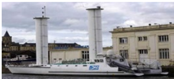
The Alcione , Jacques Cousteau's turbo sail ship, a research vessel launched in 1985, and precursor of today's rotor sail cargo ships. Image courtesy of Cousteau. org.
