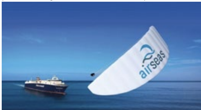
Airbus plans to equip one of its large cargo ships with the Airseas "Seawing," a sky sail that uses wind power to reduce fossil fuel costs and cut emissions. Image courtesy of AIRSEAS.
