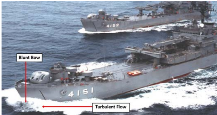
Original Hull Design of a Blunt Bow
