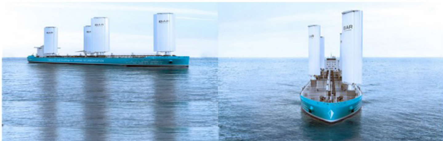
DELTAMARIN and BAR Technologies' new optimized hull design to harness wind power for 15% improvement against current fleet
