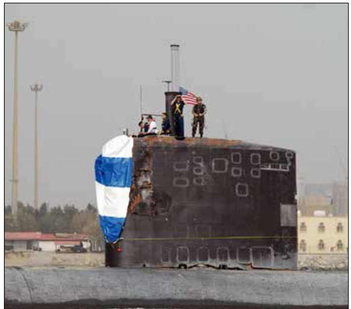
USS Hartford collided with USS New Orleans on 20-March-2009 in the Strait of Hormuz. In photo, USS Hartford in Bahrain a day after the collision.
