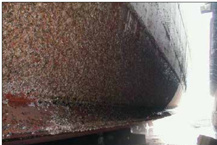
Hull fouling on a tall ship. Photo Credit: Propulsion Dynamics Inc./Marine Photobank
