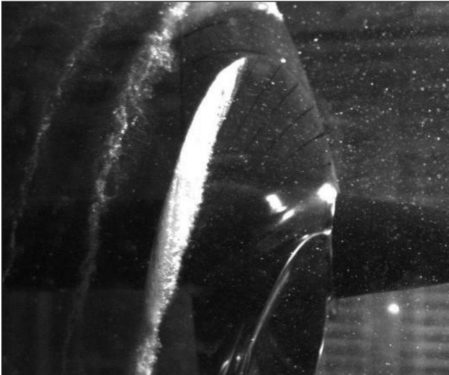
Propeller tip vortex cavitation from a modified propeller. Photo credit: Oscar Propulsion
